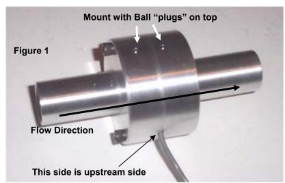
The sensor may collect liquid from condensation and oil vapors. You should periodically check by removing hoses and letting hoses drain, and tipping condensation out of both sides of sensor. When moving sensor which has accumulated liquid, be careful to keep the ball "plugs" up, so liquid can not get to this top side of the channel inside the meter.
