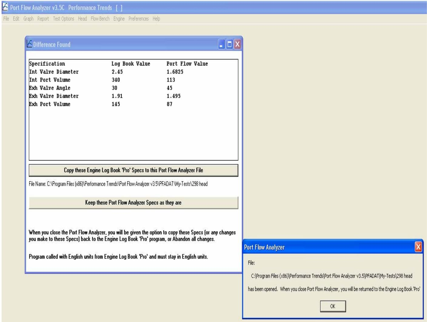
After you work with the file, or open a new file in Port Flow Analyzer, you can shut down the Port Flow Analyzer program. Then you are presented with the screen below, showing the values in the current Port Flow Analyzer file, and Engine Log Book values. This screen gives you the option to copy the Port Flow Analyzer values back to the Log Book, or just copy the file name back to the Log Book, or leave all the Log Book values unchanged.
