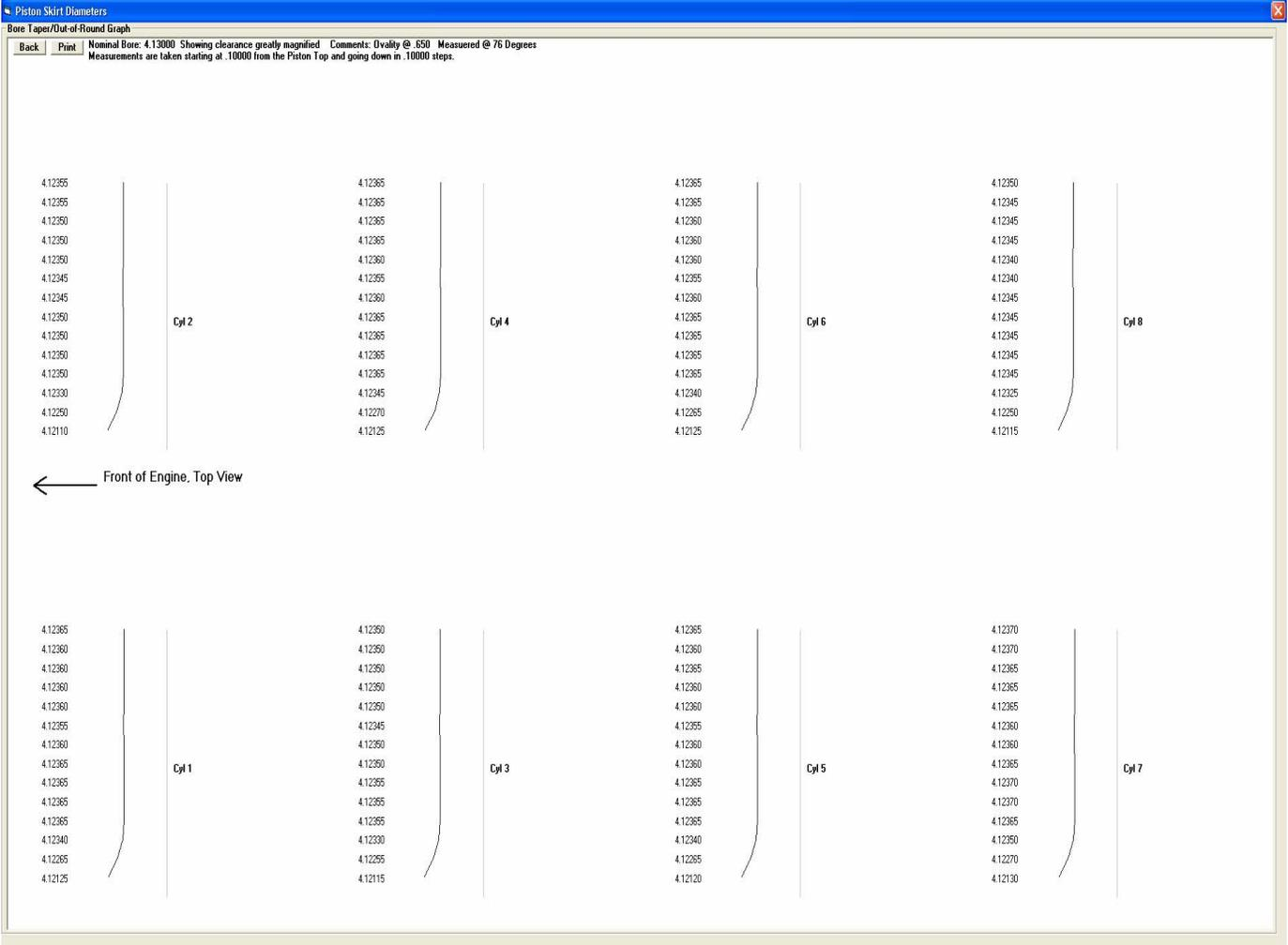
If you request Ovality (or out-of-round) readings, the 3rd tab will be for these readings taken as you go around the piston skirt in 5 degree increments. If you are in the Ovality tab you can request a Graph or Graph with Numbers., as shown below
