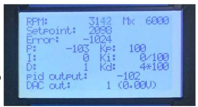
Typically the actual RPM will be slightly higher than Setpoint RPM. This allows the controller to put out a DAC out volts telling the water valve to apply more load. Typically this is with a voltage less than 2.35, like the 1.68 volts shown here.
